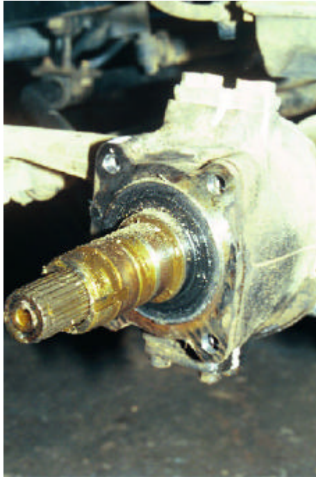
1.6 mark spindle and king pins before removal
